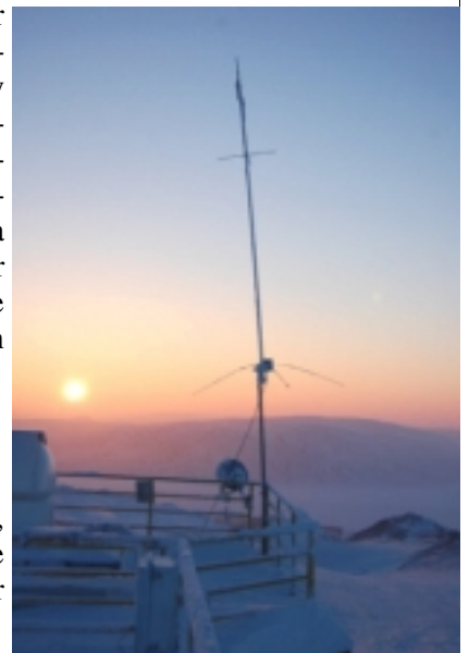
Cushcraft R5 vertical antenna at polar sunrise after surviving a 90 km/h wind storm.
