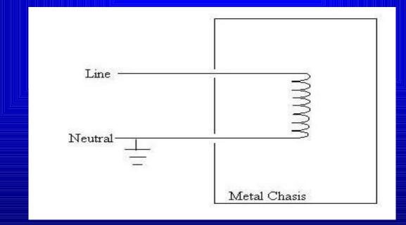
A short circuit has developed between the line or hot side of the power transformer and the chassis, thus putting the case at a potential of 115 V.
